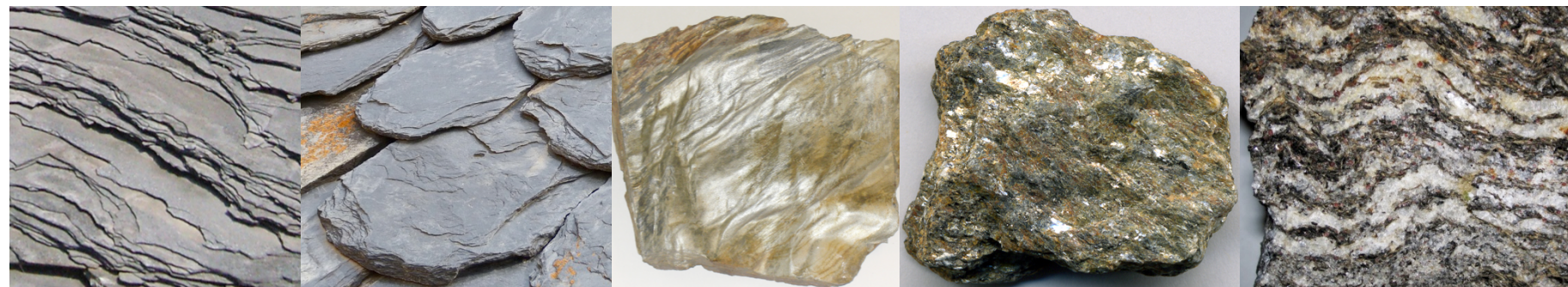
Shale (image by GorissenM) → Slate → Phyllite (image from Wikimedia Commons) → Schist (image by James St. John) → Gneiss (image by James St. John)
